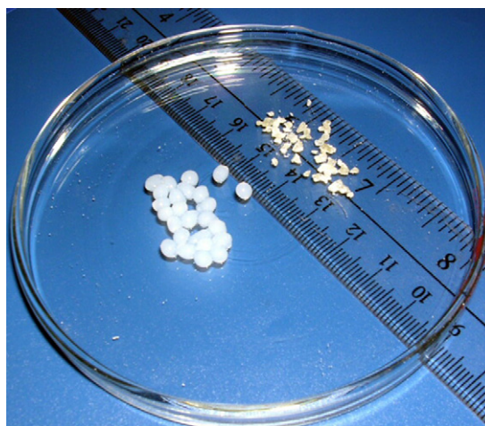
Fig. 4. Dry and wet beads prepared from formula 3 (Table 1).
